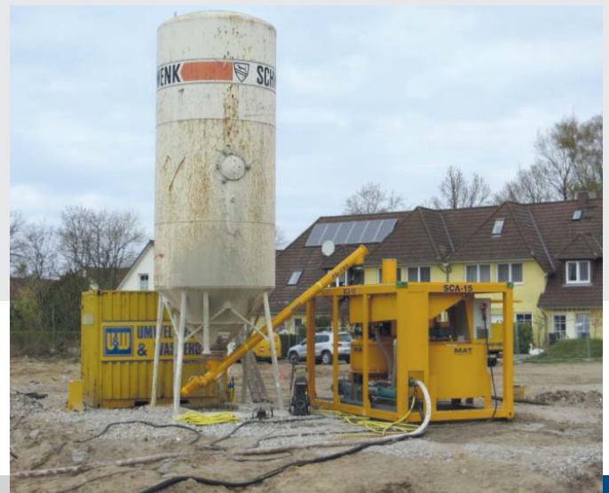
MAT SCA-15K compact mixer including pump and agitation tank
