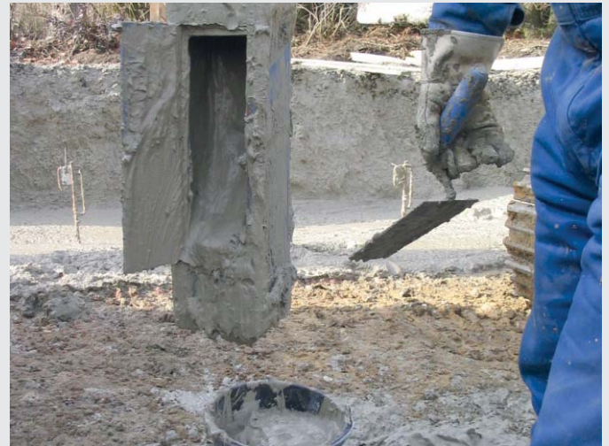
Removal of fresh samples with a sampling tool
