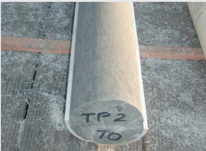
Cut-open inner plastic tube with hardened core
