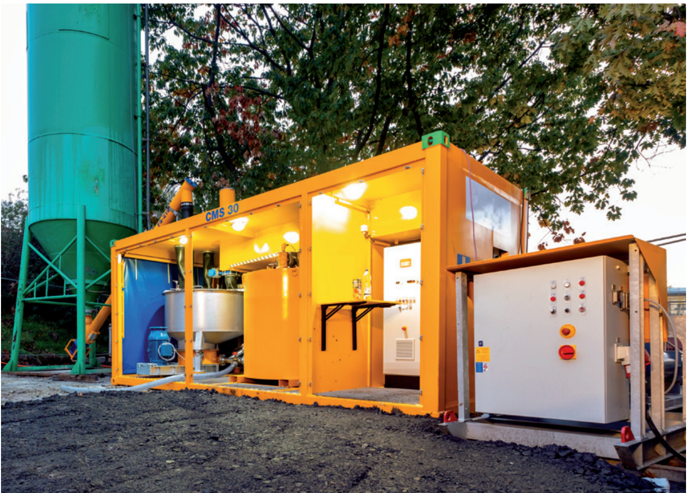
Slurry Mixing System BAUER MAT CMS-30 and slurry pump EP 14-400
