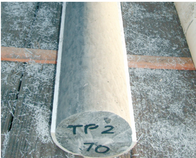
Cut-open inner plastic tube with hardened cover
