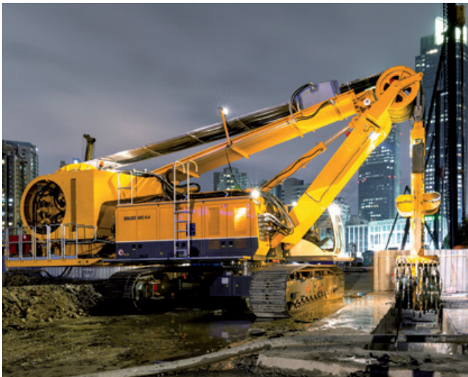
Tandem Cutter Standard on MC 64
