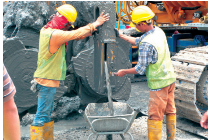
Obtaining fresh samples using a special sampling tool
