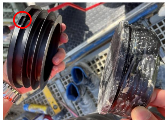
Picture 3: Concrete cover standard, one-way, new vs. old (with tape)
