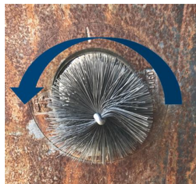
Illustration 2: Direction of rotation cleaning brush
